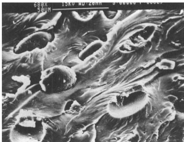
FIGURE 8 SEM micrographs for ETBN (8.3 phr) combined with an unmodified vinyl ester resin.
